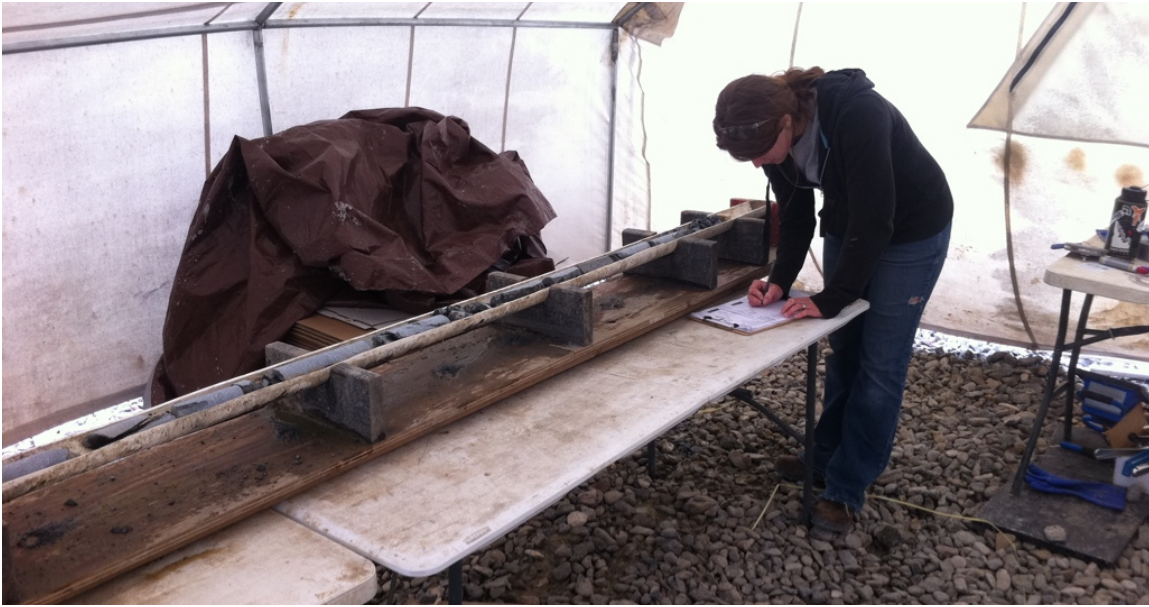
Figure A-3. Initial core logging of a core run in the PVC trough. Each core run logged for rock types, structures, and other characteristics before being boxed.
