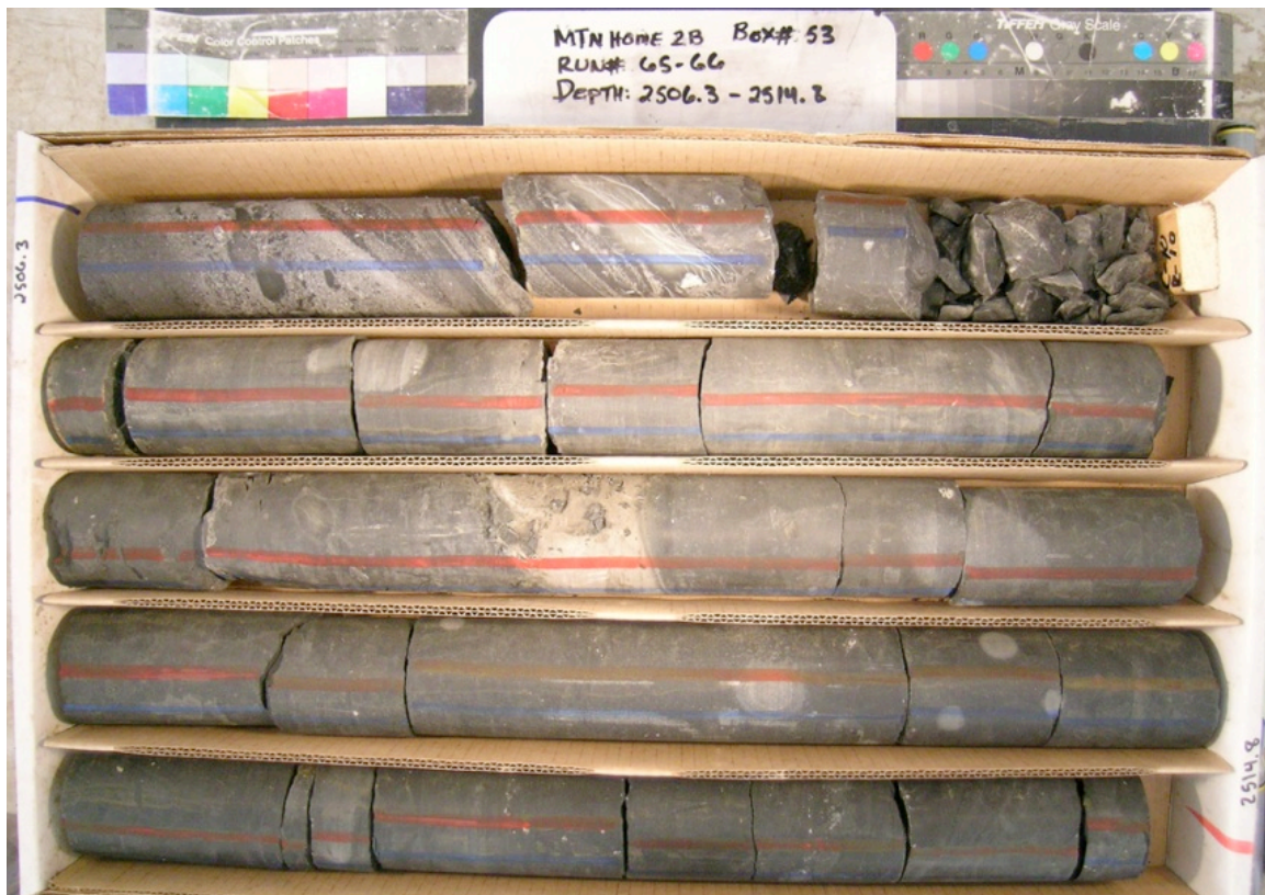
Figure A-6. Medium resolution (5 MP) photograph of boxed core, with run identification, length scale, color bars, and greyscale bars. These photos are made in Core Logging Tent onsite as core is collected, logged, and boxed.
