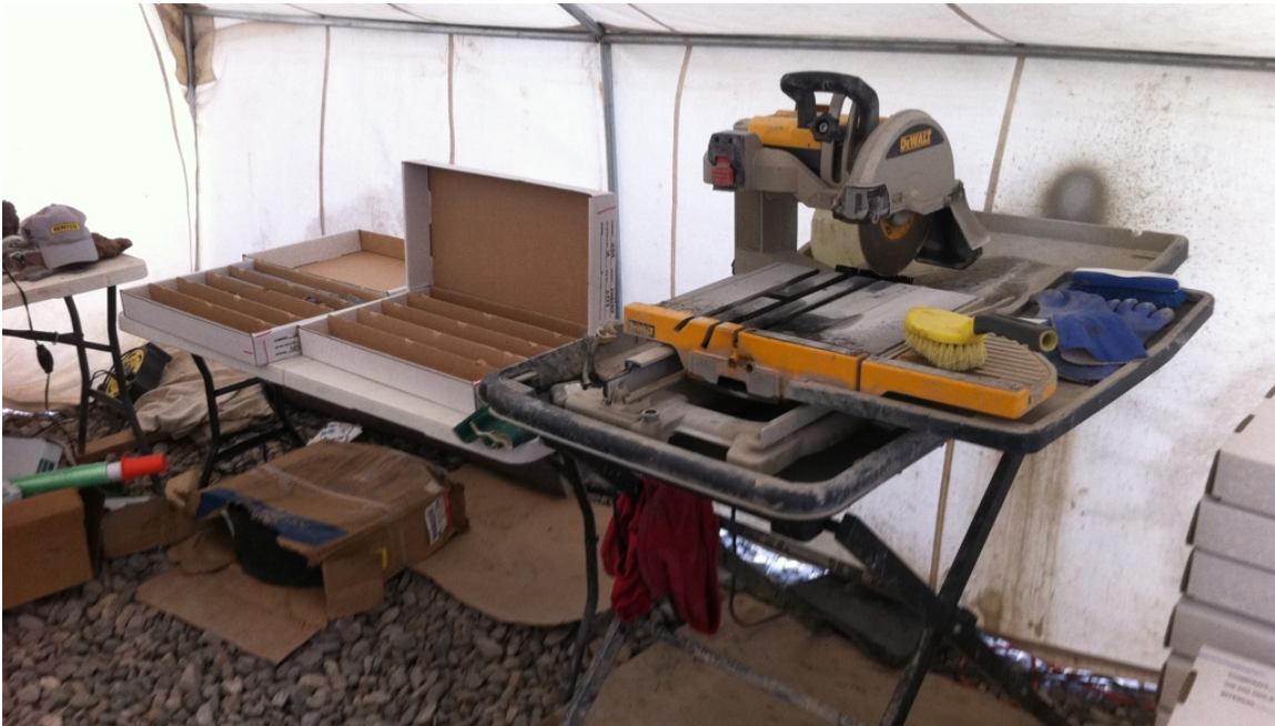
Figure A-4. Diamond table saw for cutting core. Core is cut into 2-foot lengths and boxed before being photographed and packed for shipping to the USU Core Facility.
