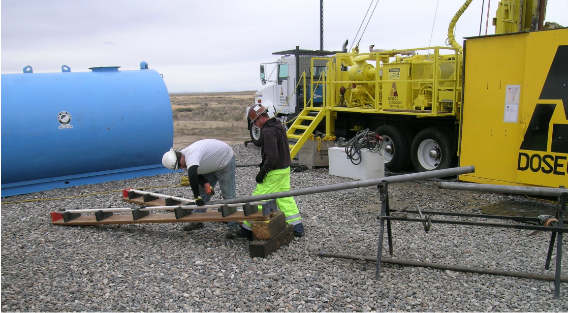
Figure A-1. Core is removed from inner core barrel by the drilling crew. Process is monitored by Science Crew to ensure that core integrity and orientation are maintained.
