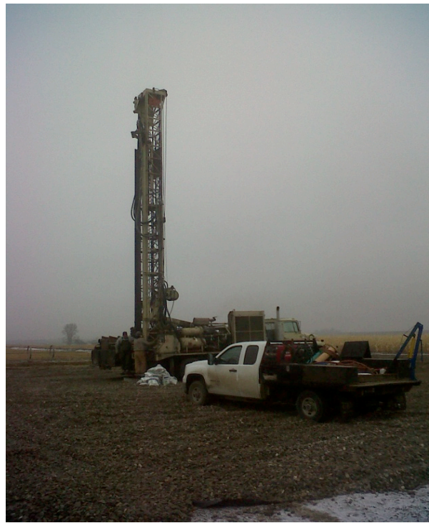
Figure 7-2. Eaton's T3W air rotary drill rig.
