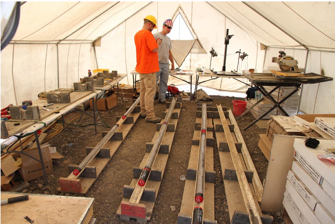
Figure A-2. Core runs in PVC troughs stored in Core Logging Tent before being logged. This sediment core was obtained in plastic core barrel liners, so it is simply capped and boxed for transport to the LacCore Facility in Minnesota.
