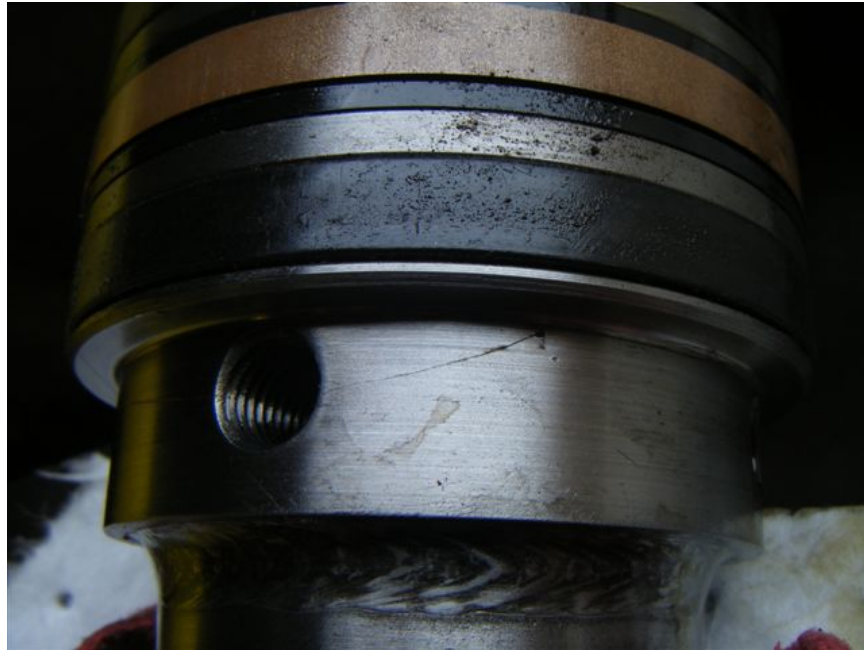
Figure 7-16. Crack perpetuated from port through seal on piston.
