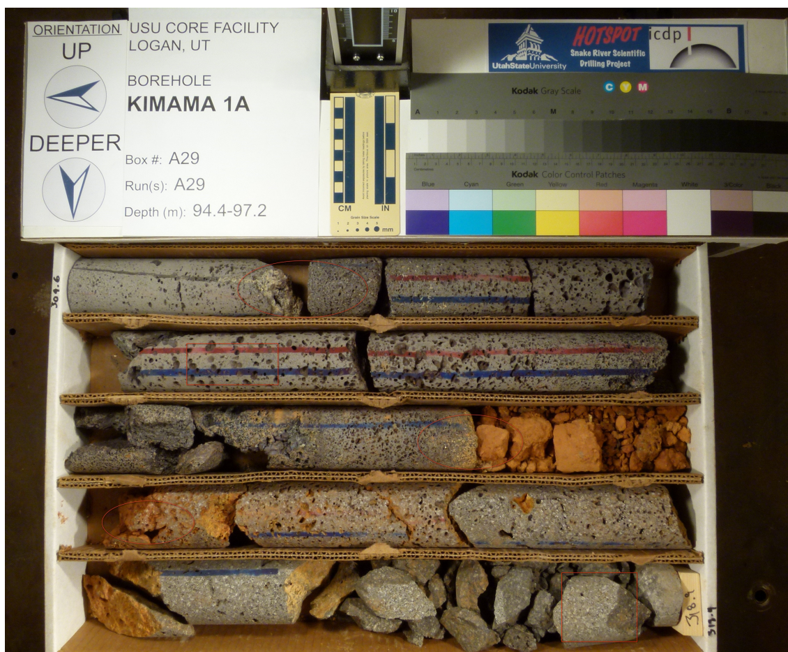
Figure A-7. Example of high resolution (15 MP RAW image) of boxed core taken at USU Core Facility. All high resolution images and core scans uploaded to the Drilling Information System database for archiving. These images are available to anyone wishing to study the core.
